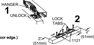
ATTACH 1121 Door Plates 2" (51mm) from door edge. (24" Door: Attach 1121 Door Plates 1/2" (12.5mm) from door edge.)
