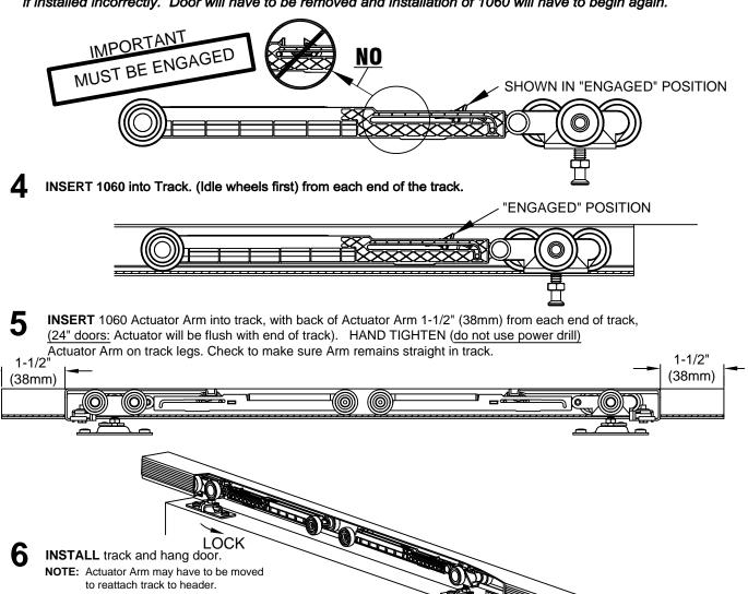
**SLOWLY** slide door toward Jambs, checking to make sure door touches Jamb, if not. Slide door away from Jamb and readjust Actuator Arm. Slowly close door again, checking to make sure soft close is working properly. Once confirmed, begin using door normally.
